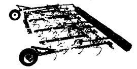
Brillion has designed a 3 pt. S-Tine field cultivator with a larger, aggressively angled 12" diameter rolling basket, a 4-bar frame that allows for either 4" or 6" tooth spacing and an adjustable coil tine leveler bar. Gauge wheels are optional.
