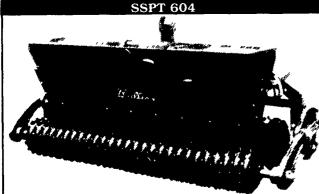
5' model has a single box with two compartments. The capacity of the front box (for chaffy seeds) is 1 1/4 bushels, the rear box (for legumes) holds 3/4 bushel. This model category 1 three point hitch.
