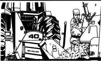
The New Holland Model 40 forage blower saves you time at the silo. This 1000-rpm blower features a 48-inch diameter hopper that centerfills silos 80 feet and higher. The Whirl-a-Feed® rotary table spins crops into the blower housing, and material gets off to a fast start up the blower pipe. Spinning action breaks up heavy clumps, and virtually eliminates plugging. There's less drag on the fan, and more efficient use of the tractor's horsepower.
