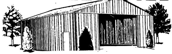
CONTRUCTION • Pressure treated posts & skirt boards • 2x4 Premium grade girts & purlins • Prefabricated clear span trusses 4' On Center • Sliding doors w/National hardware • 3°6° Prehung door • Also includes all nails, hardware, trim, plans and instructions • 29 Gauge Fabral Painted Steel Siding
