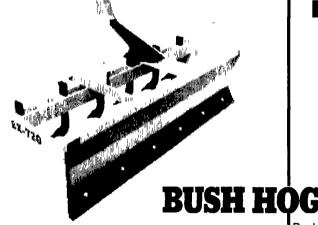
Bush Hog BX Series Box Blades scrape, back fill, back blade and scarify. These lift type implements are available in 48, 60, 65, 72 and 84-inch working widths. They feature a heavy duty A-frame, heavy duty double strap hitch, heavy 3/8-inch side plates, two high carbon heat-treated cutting edges that are reversible and replaceable and replaceable points and shanks. Shanks are easily adjustable from 0 to 3 inches. Ideal for maintaining driveways, feedlots and dozens of other uses.
