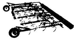
Brillion has designed a 3 pt. S-Tine field cultivator with a larger, aggressively angled 12" diameter rolling basket, a 4-bar frame that allows for either 4" or 6" tooth spacing and an adjustable coil tine leveler bar. Gauge wheels are optional.
