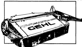
Gehl has two all-hew disc mower conditioners to cut your crop down to size, fast and easy. The DC2340 has 7 discs and a 9 foot cutting width; the DC2360 has 8 discs and a 10-1/2 foot cutting width.
