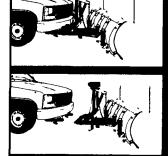
snowplow mount is quickly and easily removed from the truck when it's not being used for plowing
