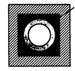
Chimtek Inner Liners are madeof volcanic pumice and hightempertature refractory cements, Its round shape provides even temperature inside flue and contributes to efficient flow of smoke and flue gasses. The volcanic pumice in Chimteck liners adds considerable insulating value.
