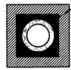
Chimtek Inner Liners are madeof volcanic pumice and hightempertature refractory cements, Its round shape provides even temperature inside flue and contributes to efficient flow of smoke and flue gasses. The volcanic pumice in Chimteck liners adds considerable insulating value.
