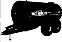
Van Dale's superior strength starts tank shell, domed heads and baffles. Tank seams overlap and are fully
