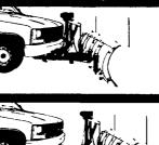
With Fisher's new Minute Mount System most of the snowplow mount is quickly and easily removed from the truck when it's not being used for plowing
