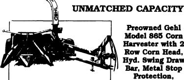
Standard equipment includes an in-head hydraulic knife and cutterbar sharpening system, electric controls, one-way shear-bolt protection system, single station cutterbar adjustment and an over-running clutch
