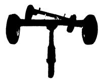
On all model wagons the steering assmblies are mounted on Taper Roller Bearings. Over 20 years field service has proven that this feature plus ball-in-socket tie rod ends assures long life and no sway trailing.
