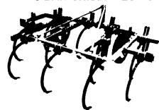
The CPP series mounted models enables you to turn short and fast... to transport easily, utilizing your tractor's hydraulic system, 7, 9, 11, 13 or 10,12,14,16 shank.
