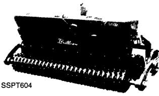
This 5' model has a single box with two compartments. The capacity of the front box (for chaffy seeds) is 1 1/4 bushels, the rear box (for legumes) holds 3/4 bushel. This model fits category 1 three point hitch.
