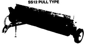
Special Features of the SS12 Pull Type are a 5 1/4 bu. meter box capacity, 5 1/4 bu. optional brome box capacity, and standard front wheel. It has a rolling width of 12'. The overall width is 15' with an approx. weight of 2547#.
