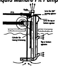
•Available 6-8-10-12 ft. •Trailer m ted mobility ·Hydraulic lift Simple controls Soil agitation
