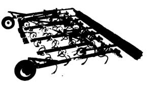
Brillion has designed a 3 pt. S-tine field cultivator with a larger, aggressively angled 12" diameter rolling basket, a 4-bar frame that allows for either 4" or 6" tooth spacing and an adjustable coil tine leveler bar. Gauge wheels are optional.
