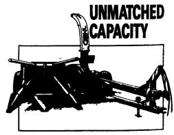
Standard equipment includes an in-head hydraulic knife and cutterbar sharpening system, electric controls, one-way shear-bolt protection system, single station cutterbar adjustment and an over-running clutch
