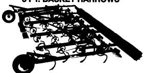
Brillion has designed a 3 pt. S-Tine field cultivator with a larger, aggressively angled 12" diameter rolling basket, a 4-bar frame that allows for either 4" or 6" tooth spacing and an adjustable leveler bar in 12', 15' and 18' sizes. Gauge wheels are optional.
