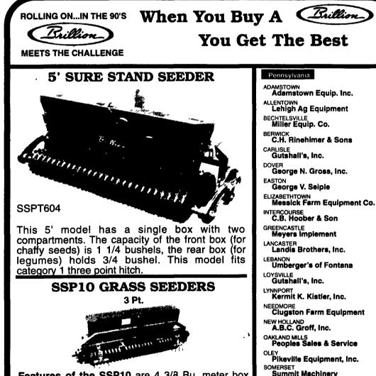
Features of the SSP10 are 4 3/8 Bu. meter box capacity, 4 3/8 brome box capacity, Standard front wheel, and a 10' rolling width. The overall width is 11'4" and approx. weight is 2018#.
