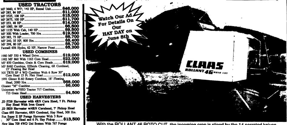
With the ROLLANT 46 ROTO CUT, the incoming crop is sliced by the 14 serrated knives, spaced 2.75" apart across the width of the intake. The resulting sliced material can be compressed to a higher density and is much easier to feed out to livestock. CLAAS ROLLANT round balers are a cost effective investment thanks to their output, reliability and ease of maintenance. Their versatility also helps to keep them in action for many months of the year.
