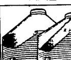
High Capacity 40° roof (left) allows more storage and stays cleaner than conventional 30° roof (right)
