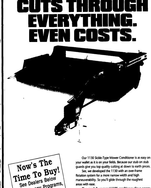
Plus, our fully engaged 110" conditioner allows aggressive hay conditioning for faster drying. It'll also clear itself of crop jams with its own automatic plug release.
