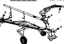
Gear box oil bath protected by a > greaseable 3 seals mechanism on each shaft. AVAILABLE WITH MULTIPURPOSE OPTION TO ALSO CLIMB INTO CONCRETE PITS UP TO 14' DEEP
