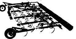
Brillion has designed a 3 pt. S-Tine field cultivator with a larger, aggressive angled 12" diameter rolling basket, a 4-bar frame that allows for either 4" or 6" tooth spacing and an adjustable coil tine leveler bar. Gauge wheels are optional.
