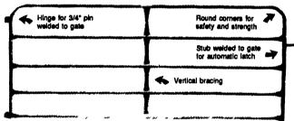
Standard Heights For Gates & Fencing: (38" High - 4 Bar) (48" High - 5 Bar) (54" High - 6 Bar)
