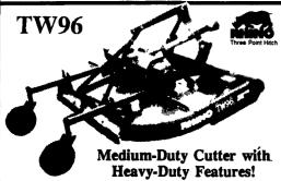
96" Cut; 120 HP Center Gearbox; 90 HP Outboard Gearboxes; Pan Blade Carriers; Updraft Blades; Cat. 4 Driveline; Slip Clutch Protection; Lift or Pull-Type; 540 or 1000 RPM; Replaceable Skid Shoes; Rated for 2" Diameter Material; Safety Deflectors
