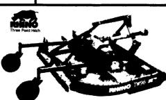
Binkley & Hurst Has A Quality **TW120** Rhino Cutter In Stock For You Now! Pull-Type; 10-Gauge Deck; 1/4"x10" Side Skirts; Replaceable Skid Shoes; Rated for 2" Diameter Material; Safety
