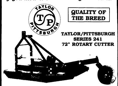
Quality was bred into the 240 Series Rotary Cutters by the great reputation of Taylor Way and Pittsburgh Quality Equipment. The 240 Series come standard with stump jumper and laminated gauge wheel. Also standard is an 11 gauge deck and shearbolt or an optional slip clutch. The quality and price of the 240 Series Mower make it the most productive tool you'll ever have on your farm.
