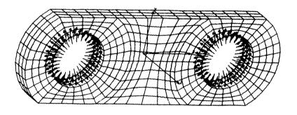
The Marathon cutter chain features sidebars with full round bushing design for improved stress distribution, and a full contact press fit between the bushing and sidebar.
