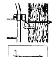
The through-post gate hanger, from Gallagher Power Fence, Inc., eliminates the problem of the shaft turning in the post by having a second shaft, without threads, which penetrates the post below and parallel to the primary, threaded shaft.
