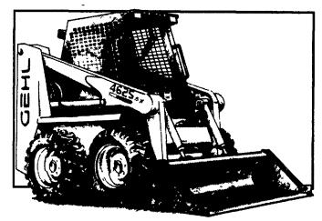
Precise bucket and drive control is easy with Gehl's exclusive Load-Trak T-bar hand controls. Optional hand/foot controls also available,
