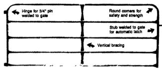
Standard Heights For Gates & Fencing: 8" High - 4 Bar) (48" High - 5 Bar) (54" High - 6 Bar) (38" High - 4 Bar)
