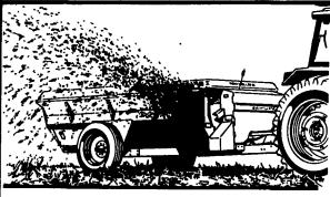
New Holland side delivery spreaders handle a variety-of materials poutity free stall and guiter manure from bean cleaners - even most pen packed manure. You get precise control over the amount of material per acre. Spreading rates are hydraulically con trolled, providing uniform spread patterns.
