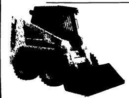
5625 56 HP Diesel 1,700 lb. SAE Operating Capacity
