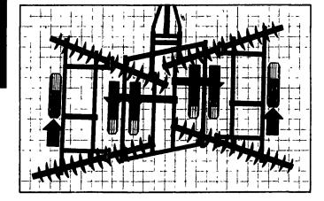
This special wheel arrangement saves fuel by helping to prevent gouging.
