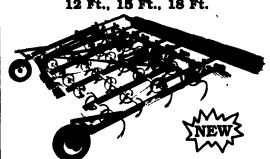
Brillion has designed a 3 pt. S-Tine field cultivator with a larger, aggressively angled 12° diameter rolling basket, a 4-bar frame that allows for either 4" or 6" tooth spacing and an adjustable coil tine leveler bar. Gauge wheels are
