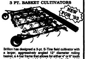
spacing and an adjustable leveler bar in 12', 15' and 18' sizes. The distance between the four bars has been increased for the best trash flow in the industry. Gauge wheels are optional.
