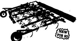
Brillion has designed a 3 pt. S-Tine field cultivator with a larger, aggressively angled 12" diameter rolling basket, a 4-bar frame that allows for either 4" or 6" tooth spacing and an adjustable leveler bar in 12', 15' and 18' sizes. Gauge wheels are optional.
