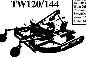
Performance and Durability for Larger Acreages! 120" and 144" Cut; 120 HP Center Gearbox; 100 HP Outboard Gearboxes; Pan Blade Carriers; Updraft Blades; Cat. 4 Driveline with Slip Clutch Protection; 540 or 1000 RPM; Lift or Pull-Type; 10-Gauge Deck; 1/4" x 10" Side Skirts; Replaceable Skid Shoes; Rated for 2" Diameter Material; Safety Deflectors Standard.
