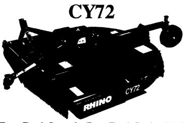
Extra Tough Cutter for Extra Tough Cutting Jobs! 72" Cut; 540 or 1000 RPM; CAT II Heavy-Duty Three-Point Hitch; 140 HP "Rhino-Built" Gearbox (1000 RPM); Cat. 4 Shielded Driveline; Slip Clutch Protection; Heavy-Duty Pan Blade Carrier; 3/16" Deck; 1/4" x 9" Side Skirts; 1/2" x 4" Updraft or Flat Blades; Rated for 4" Diameter Material; Safety Deflectors Standard.
