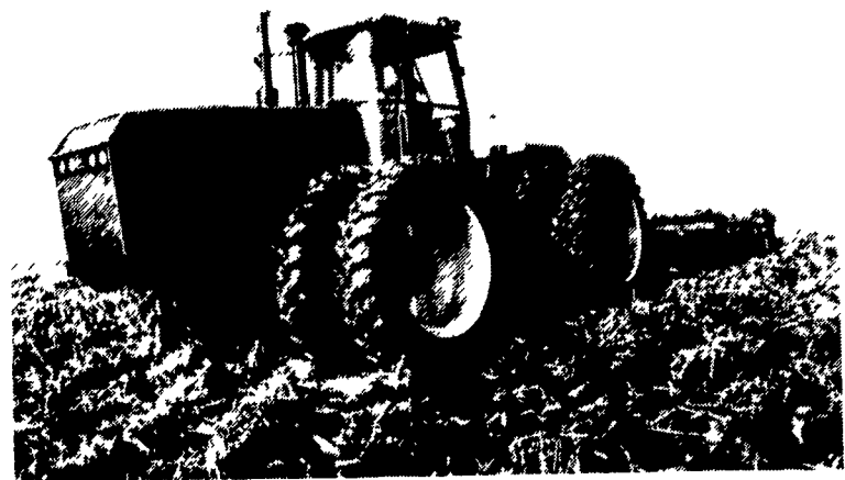
The 250-HP John Deere 8570 is one of four new 70 Series 4-wheel-drive tractors which also include the 300-hp 8770, 350-hp 8870, and 400-hp 8970. The tractors feature increased engine performance, enhanced operator comfort, and improved ease of service.
