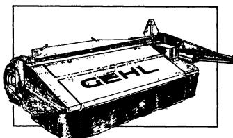
Gehl has two all-new disc mower conditioners to cut your crop down to size, fast and easy. The DC2340 has 7 discs and a 9 foot cutting width; the DC2360 has 8 discs and a 10-1/2 foot cutting width.
