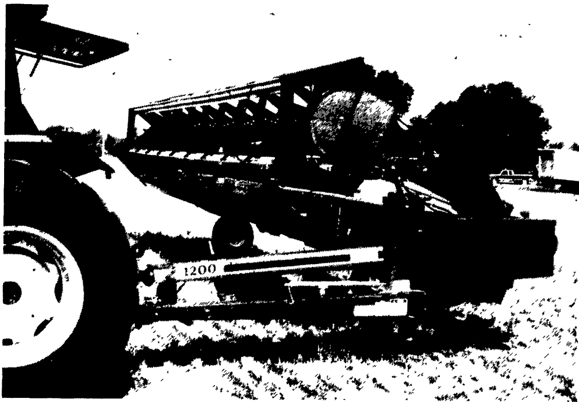
Available in four different header units of 21-feet, 25-feet, 30-feet, and 35-feet, the PT 1200 is equipped with a variable speed reel and an adjustable swath opening as standard equipment.
