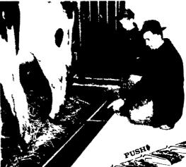
Malleable iron paddles attached to the bar open across the gutter to move manure toward the spreader on the forward stroke.
