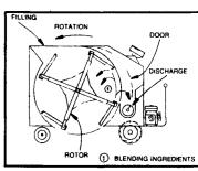
The exclusive mobile Rovibec mixer, with adjustable rotating beaters, provides a consistently uniform blend of all ingredients, from the first to the last ration.
