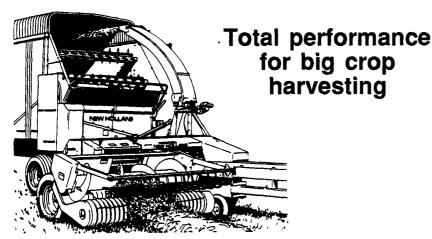
You get total performance when you harvest your crops with a Model 900 forage harvester. Total performance begins at the cutterhead. The 12 knives of the 21-inch cutterhead give you uniformly cut, high-quality forage. Other features on the "900" include:
