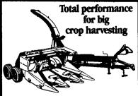
You get total performance when you harvest your crops with a Model 900 forage harvester. Total performance begins at the cutterhead. The 12 knives of the 21-inch cutterhead give you uniformly cut, high-quality forage. Other features on the "900" include:
