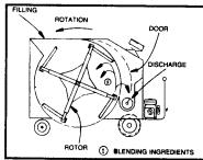
The exclusive mobile Rovibec mixer, with adjustable rotating beaters, provides a consistently uniform blend of all ingredients, from the first to the last ration.
